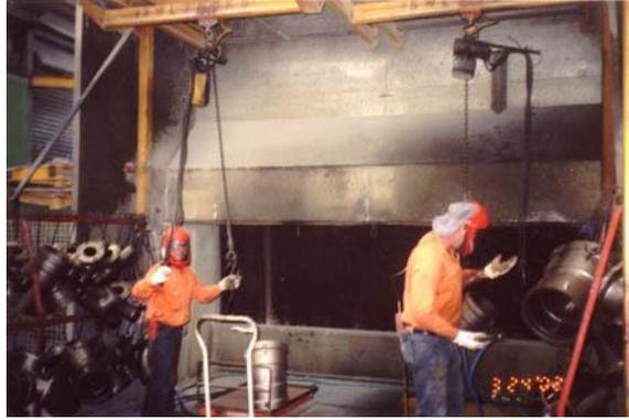
The pictured spray booth is used for solvent and water based paint primers and is fitted with a wet scrubber, using triple<sup>7</sup> Odour Control or Odour-Ex.
